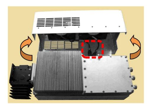
Figure C-9. Fan Shroud Removal
