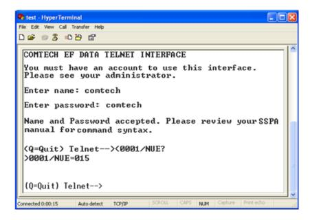
Figure 4-2. Telnet Interface Example – HyperTerminal
