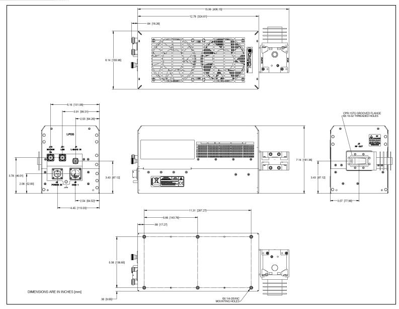
Figure 1-11. LPOD PS 1.5 C-Band Dimensional Envelope (AC Option)
