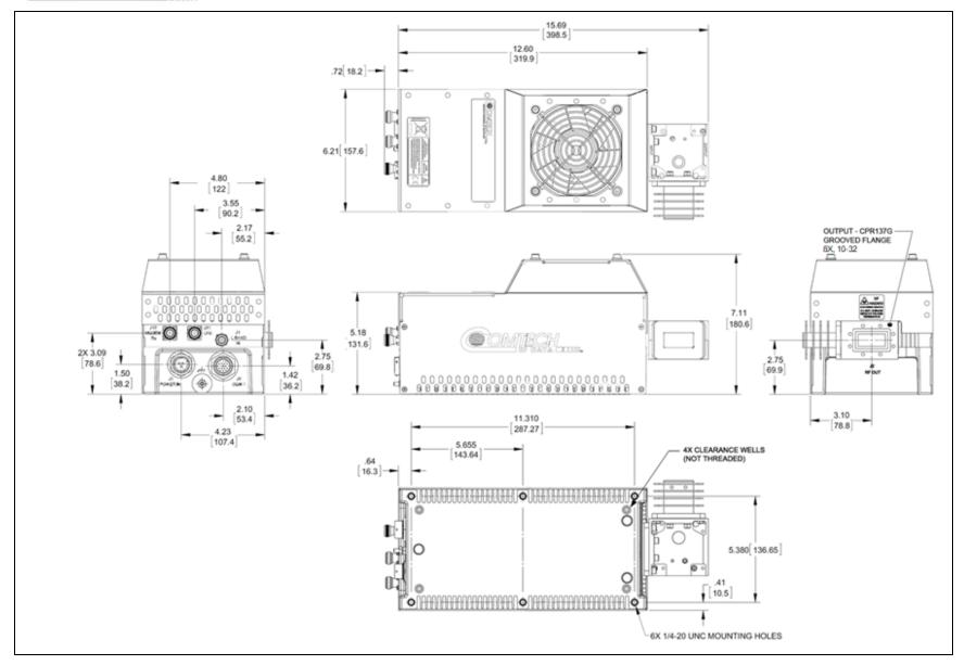
Figure 1-6. LPOD PS 1 C-Band Dimensional Envelope
