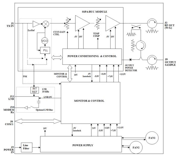
Figure 1-3. LPOD PS 2 Block Diagram
