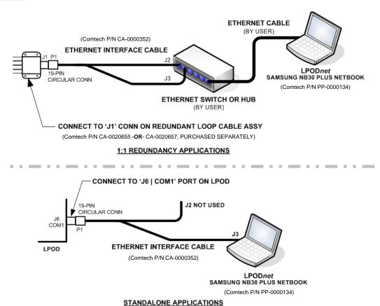
Figure A-1. Ethernet-based M&C using Comtech Kit KT-0000203
