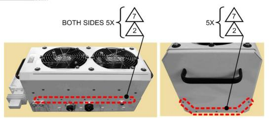
Figure C-13. LPOD PS 2 Shroud Screw Locations
