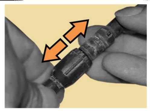
Figure C-15. Fan 1 / Fan 2 Power Supplies Disconnection
