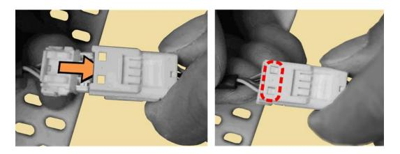
Figure C-7. Fan Power Supply Reconnection
