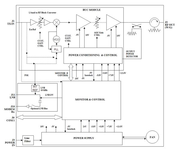
Figure 1-2. LPOD PS 1 and PS 1.5 Block Diagram
