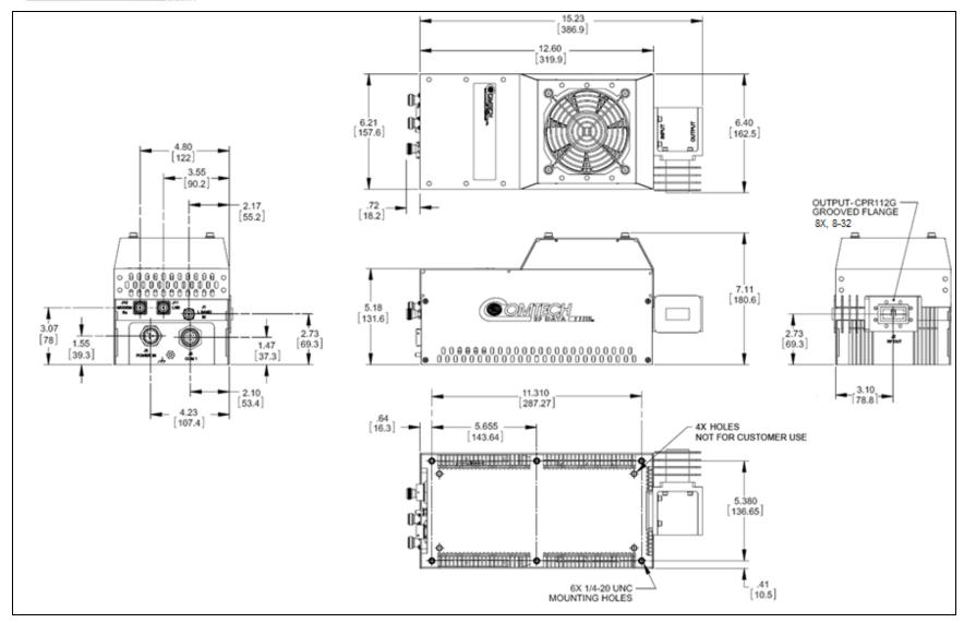
Figure 1-7. LPOD PS 1 X-Band Dimensional Envelope
