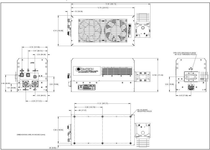
Figure 1-10. LPOD PS 1.5 C-Band Dimensional Envelope (DC Option)
