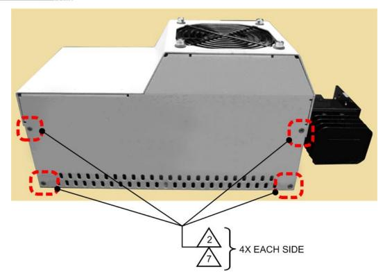
Figure C-3. LPOD PS 1 Shroud Screw Locations
