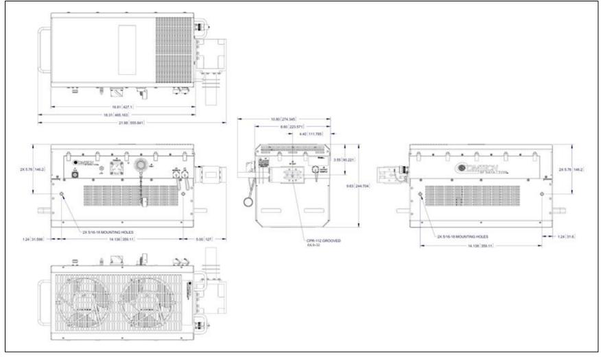
Figure 1-15. LPOD PS 2 X-Band Dimensional Envelope
