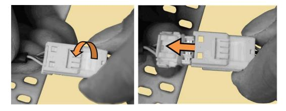
Figure C-5. Fan Power Supply Disconnection
