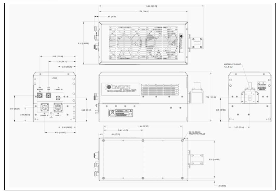
Figure 1-13. LPOD PS 1.5 Ku-Band Dimensional Envelope
