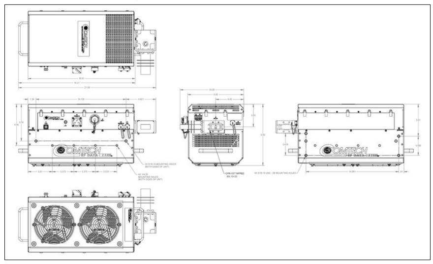
Figure 1-14. LPOD PS 2 C-Band Dimensional Envelope
