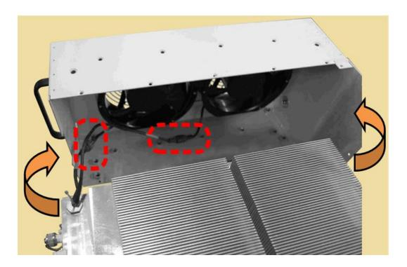
Figure C-14. Fan Shroud Removal
