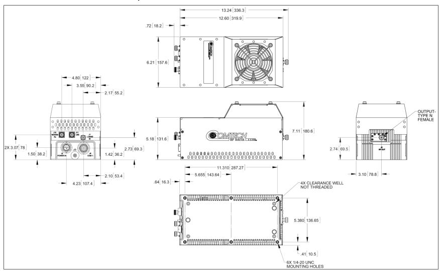
Figure 1-4. LPOD PS 1 C-Band Dimensional Envelope (Coax Output)
