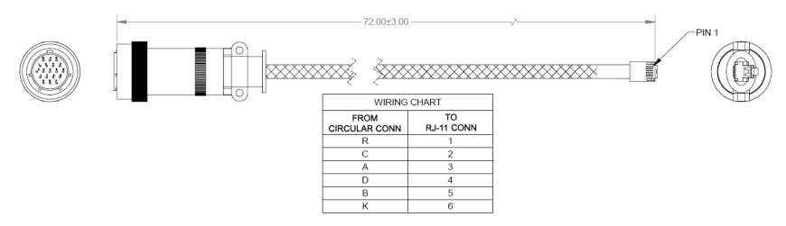
Figure B-1. Serial Interface Cable (Comtech P/N CA-0020526, part of KT-0020518)
