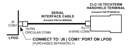
Figure 3-1. Standalone or Redundant Serial Connection
