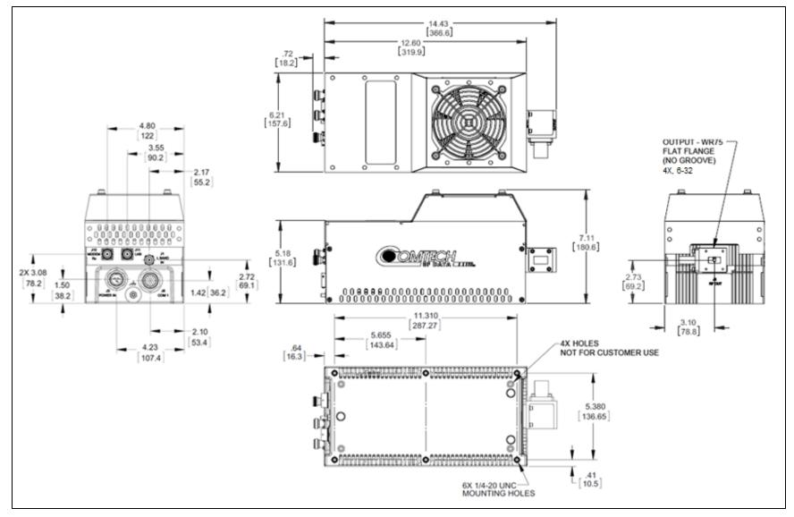
Figure 1-8. LPOD PS 1 Ku-Band Dimensional Envelope
