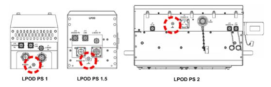
Figure 2-7. Ground Connector Locations
