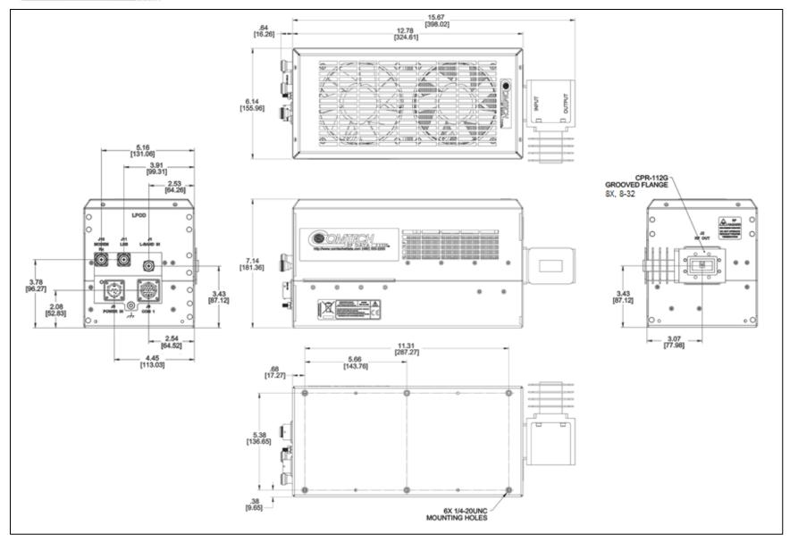
Figure 1-12. LPOD PS 1.5 X-Band Dimensional Envelope
