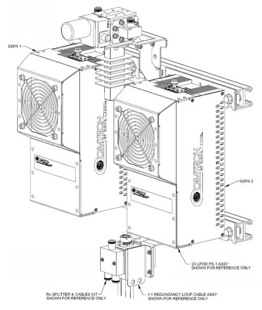
Figure A-13. KT-0000104 LPOD PS 1 C-Band 1:1 Redundancy Kit Example – Assembled Isometric View
