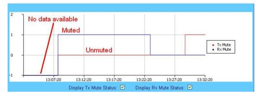
This graph displays the mute state (i.e., bias tee switch state as open = *muted*, or through path = *unmuted*) for the Tx Mute (red line) and the Rx Mute (blue line). Note that:
