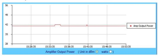
This graph displays the unit's output power with 1dB resolution. You may set this information to display as **dBm** (the default setting) or **watts.** The graph will update dynamically after the next polling cycle (every five seconds).
