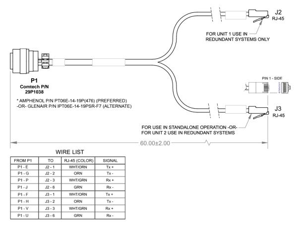
Figure B-2. Ethernet Interface Cable (Comtech P/N CA-0000352, part of KT-0000203)
