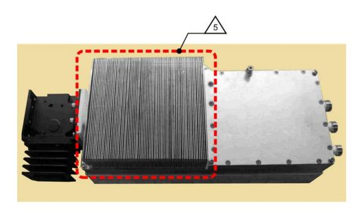
Figure C-11. LPOD PS 1.5 Heat Sink Location
