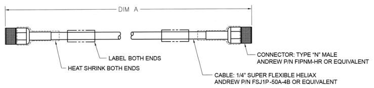
Figure B-7. 1/4" Heliax Coaxial Cable (Comtech P/N CA/3722-X)
