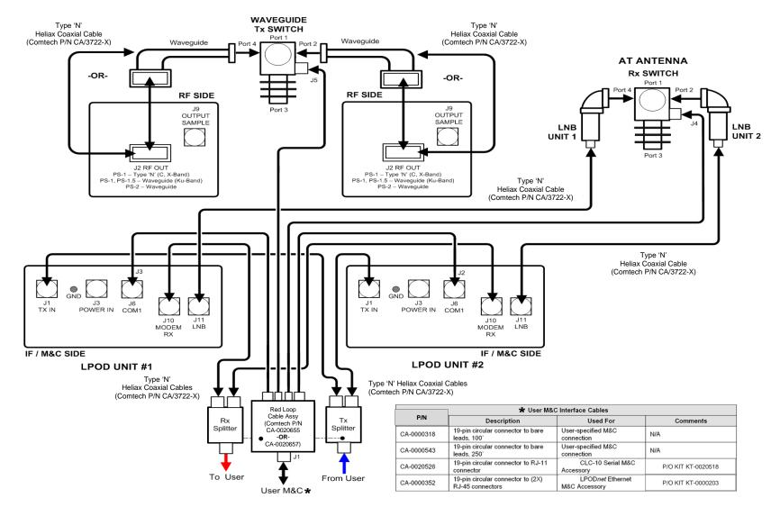
Figure A-3. Typical LPOD 1:1 Redundancy System Cabling Schematic
