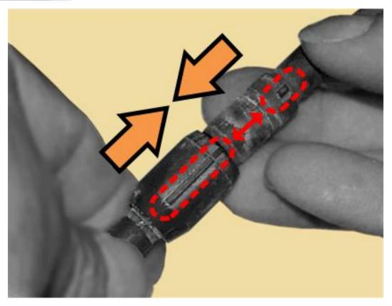
Figure C-17. Fan 1 / Fan 2 Power Supplies Reconnection
