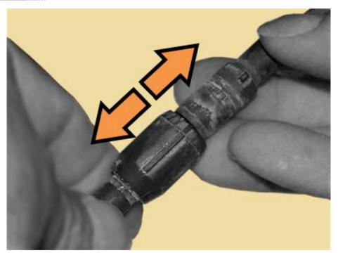
Figure C-10. Fan 1 / Fan 2 Power Supplies Disconnection
