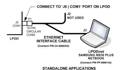
Figure 3-2. Standalone or Redundant Ethernet Connection
