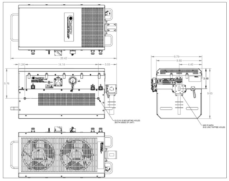
Figure 1-16. LPOD PS 2 Ku-Band Dimensional Envelope
